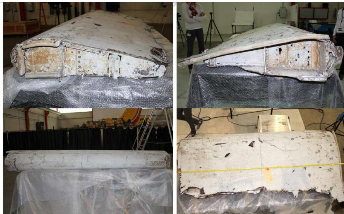
Figure 2 – Dorsal appearance of the flaperon, domed section, from left to right and top to bottom: left side, right side, front, dorsal-posterior view (small colonies of barnacles on the right).
