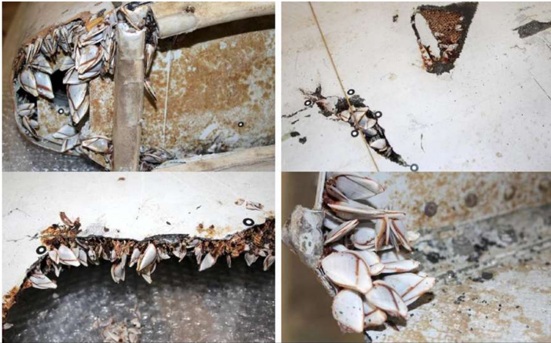
Figure 1 - Fastening of barnacles more on the rough portions of the flaperon, from left to right and top to bottom: front left edge with the largest barnacles, small colonies on scratched areas of the dorsal side, colonies attached to the bare composite on the back edge, colony on a metal corner.
